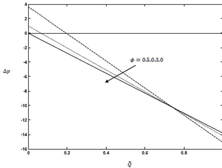
Fig. 7: The variation of pressure rise  $\Delta p$  with  $\bar{Q}$  for different values of  $\phi$  with  $\lambda_1 = 0.3$  and  $Da = 0.1$ .
