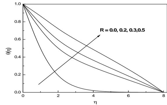
**Figure-6(b):** Temperature profiles with different  $R$
