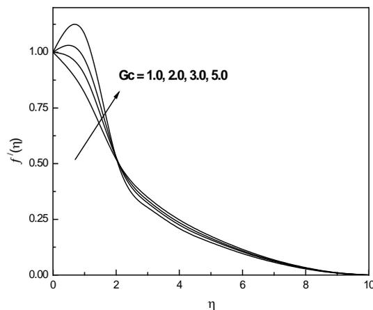
**Figure-2:** Velocity profiles with different Gc
