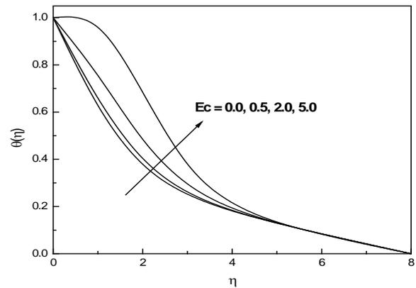
**Figure-8(b):** Temperature profiles with different  $Ec$
