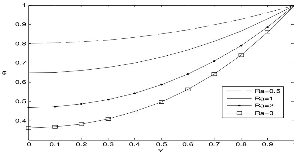
Fig (9): Graph of temperature profiles for different values of Radiation Parameter 'Ra'.
