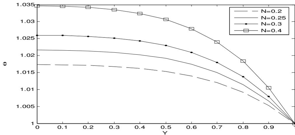
**Fig(6):** Graph of temperature profiles for different values of the dimensionless number measuring the buoyancy force 'N'.
