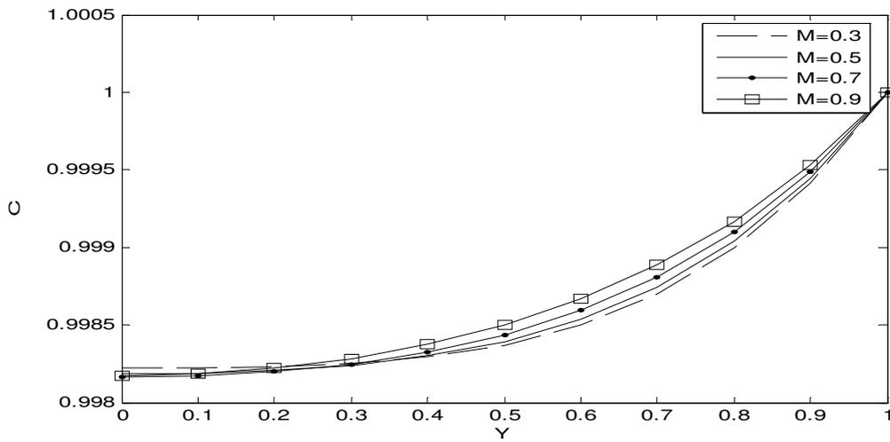
Fig(3): Graph of concentration profiles for different values of Hartmann number 'M'.
