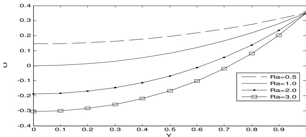
Fig (12): Graph of velocity profiles for different values of Radiation Parameter 'Ra'
