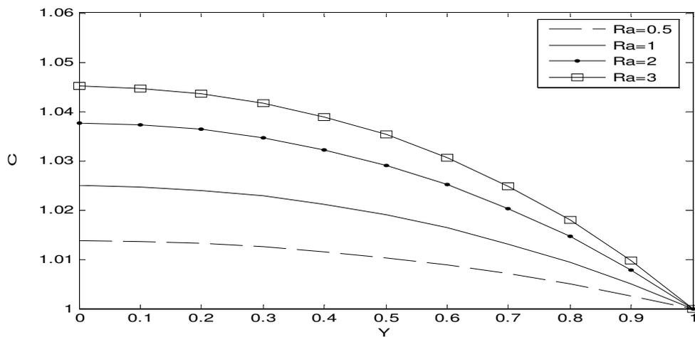
Fig(5): Graph of concentration profiles for different values of Radiation Parameter 'Ra'.
