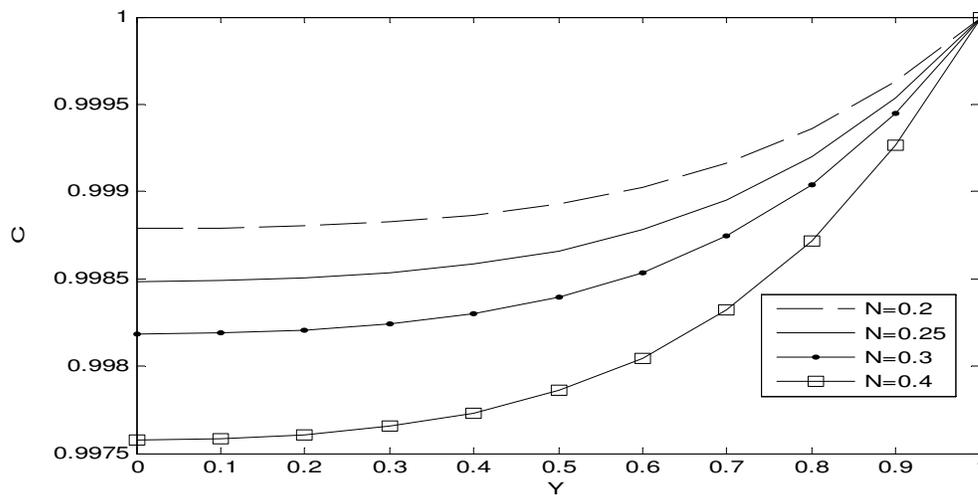
Fig(1): Graph of concentration profiles for different values of the dimensionless number measuring the buoyancy force 'N'.
