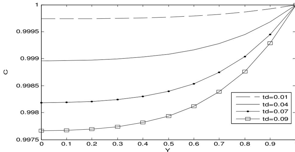
Fig(2): Graph of concentration profiles for different values of thermal diffusion number 'td'.
