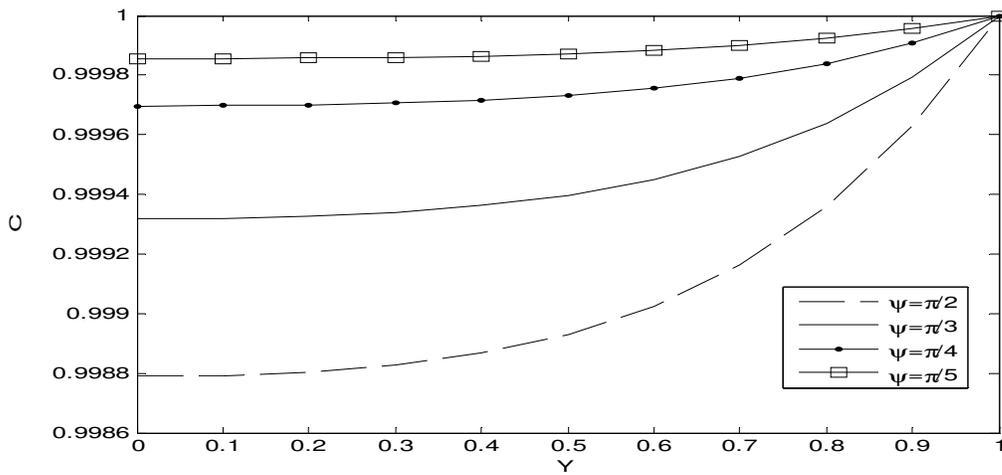
Fig(4): Graph of concentration profiles for different values of the angles that the plates make the horizontal  $\psi$ .
