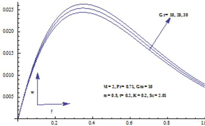
Figure-12: Velocity profile  $w$  for different values of  $Gr$ .
