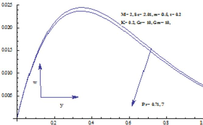
Figure-13: Velocity profile  $w$  for different values of  $Pr$ .
